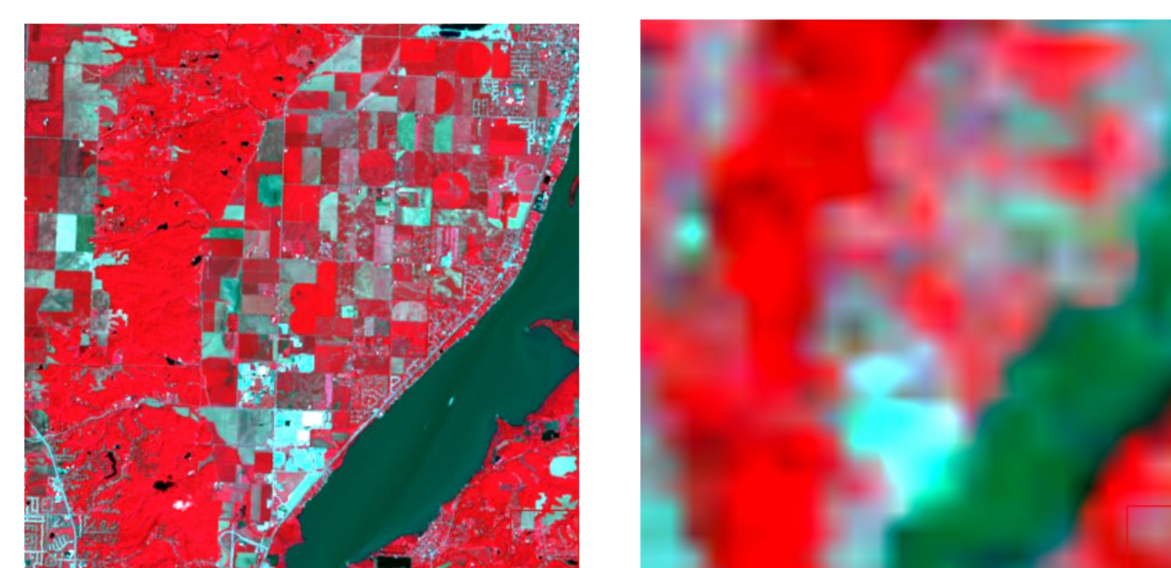
A subset of our study site in Landsat-8 OLI 30-meter imagery (left) and MODIS 500-meter imagery (right); both images acquired on June 27, 2017.
